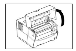
Lift the Developer Unit together with the Toner Container out of the printer.
